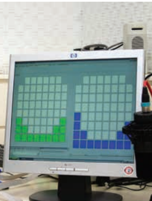
Left: EPG therapy set up. The target articulation is displayed on the right hand side of the computer screen. The left hand pattern is the client's attempt to match the target.
